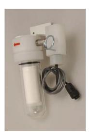
Inert PVDF material is used in constructing the water slip sensor to prevent absorption of relevant gases. The water slip sensor is often used in conjunction with the Baldwin<sup>™</sup>-Series in-line sample filter assembly (3KFA-001), which is used on all Wall/Rack mounted and Testers' Choice portable sample conditioning systems to provide fine particulate filtration.
