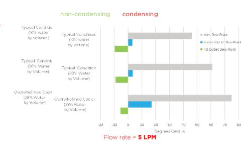
In the worst case scenario where a thermoelectric cooler completely fails, the PD-Series Gas Dryer, maintains an outlet dew point well below ambient levels helping to prevent condensation and avoid complete shutdown of the line until repairs can be made.
