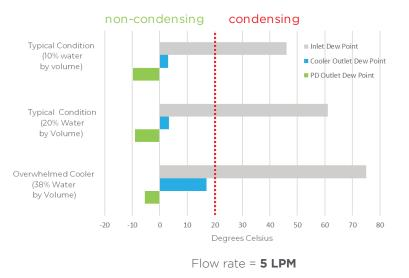
In the worst case scenario where a thermoelectric cooler completely fails, the PD-Series Gas Dryer, maintains an outlet dew point well below ambient levels helping to prevent condensation and avoid complete shutdown of the line until repairs can be made.
